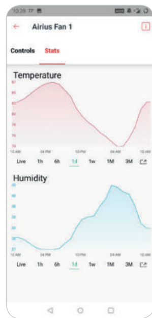
The stats tab shows temperature and humidity at the device over various periods of time. You can export this information as a csv from this view.
